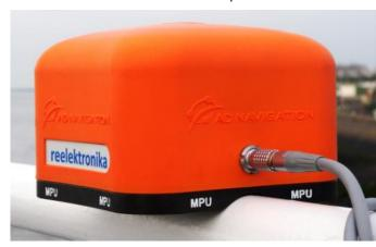
A special small portable battery-powered eDLoran receiver has been designed for use by pilots. It receives eLoran signals and sends these via bluetooth to the pilot's laptop which also receives the eDLoran corrections via the mobile network. The laptop processes the corrections and depicts the result on the electronic map together with the GPS and/or eDLoran positions. The red marker on the map below depicts the eDLoran position while the center of the ship is the 'true' GPS-RTK position.
