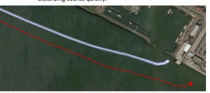
The resulting accuracy can be impressive as is shown above. The red track is eLoran without ASF and eDLoran
