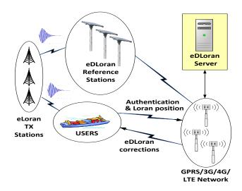
The intelligence of the **eDLoran** network is at the server in a protected area. All reference stations send their measurements to this server which therefore can calculate the best possible corrections for the user at its current location. It further allows to monitor all reference stations as part of the integrity control of **eDLoran**.
